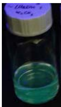
Fig.2 Vial containing a batch of SiNCs functionalized with amines in MeOH under UV light
